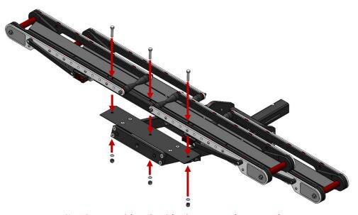
Note: Do not overtighten. Overtightening may cause damage to rack.
