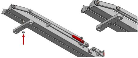
Note: Position Roof Rack Clamps to accommodate existing crossbars.
