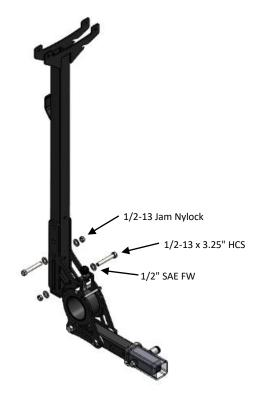
To adjust rack height, loosen lower bolt, remove top bolt, adjust to desired position, reinstall top bolt and tighten lower bolt.
