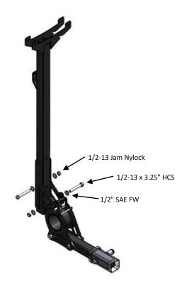
• To adjust rack height, loosen lower bolt, remove top bolt, adjust to desired position, reinstall top bolt and tighten lower bolt.
