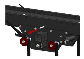
• Slide out Ramp from Tray cavity and engage end cutout with Ramp Rod.
