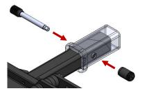
Using supplied Wrench, tighten Anti-Wobble Tensioner clockwise until Rack is stable in receiver. If loose after tightening, slightly lift Rack and continue tightening until stable.
