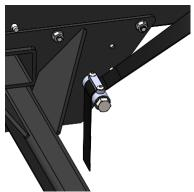
Note: If installed correctly, Straps will be of same tension when fully opening Bent Arm Assembly.
