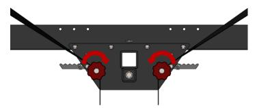
Reinstall Pins in both Driver and Passenger Bent Arm Assemblies.
