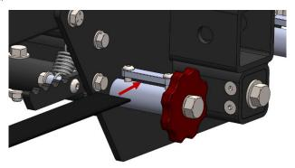
Pull back Strap through gap between Strap Clamp and Mandrel. Tension Strap by pulling slack and tighten 1/4"-20 Button Head Screws.
