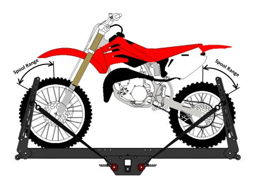
Note: Spools must contact tires within specified range. Bike is not secured on Rack if Spools are located outside of specified range.
