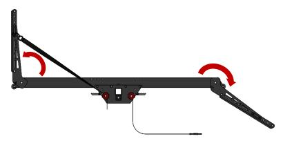
Pull Ramp Detent Pin from center of Tray.
