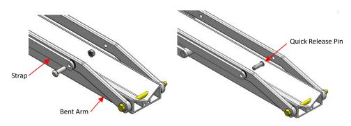
Install Quick Release Pin through Bent Arm, Spacer, and Strap.
