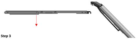
Roll Bike up V Style Ramp Long and onto Rack Trays. Use Bent Arm, opposite of ramp, to stabilize bike while loading.
