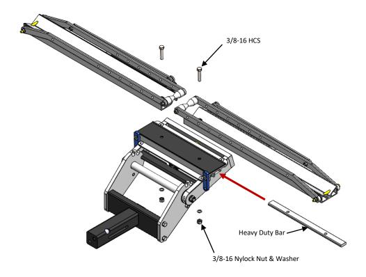
Note: Periodically tighten fasteners to ensure secure connection.
