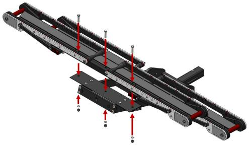
Note: Do not overtighten. Overtightening may cause damage to rack.
