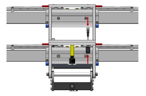
Note: Periodically tighten Security Bolts to ensure secure connection.
