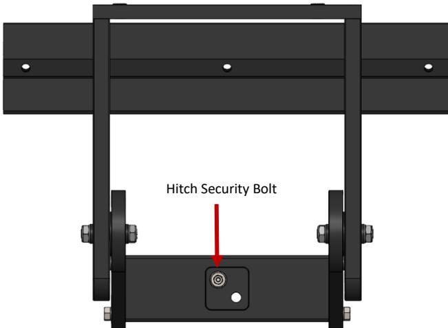
**Note:** *Do not tighten Security Hitch Bolt if Hitch Bar is not inserted into receiver.*
