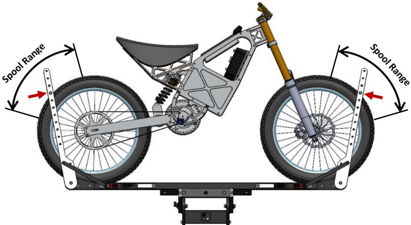
**Note:** *Spool must contact tire within specified range. Bike is not secured in rack if spool is located outside of specified range.*
