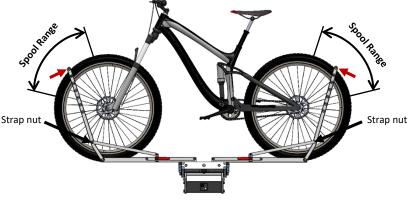
Note: Spool must contact tire within specified range. Bike is not secured in rack if spool is located outside of specified range.
