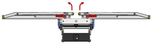
Note: Do not move Bent Arms up without lifting Red Lever.
