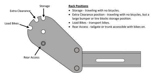
Note: In rear access position, Black Bar will not lock into place. Not for transporting.
